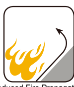
Reduced Fire Propagation NF C32-070-2.2(C1) IEC60332-3-24 EN50266-2-4
