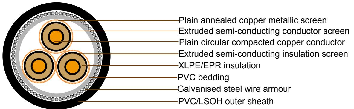
**CONDUCTOR:** Plain circular compacted copper to AS/NZS1125
