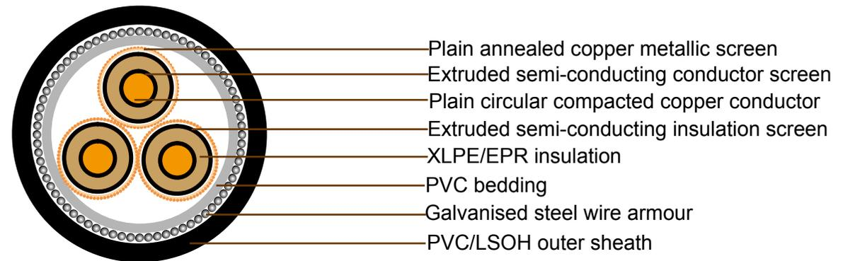
**CONDUCTOR:** Plain circular compacted copper to AS/NZS1125
