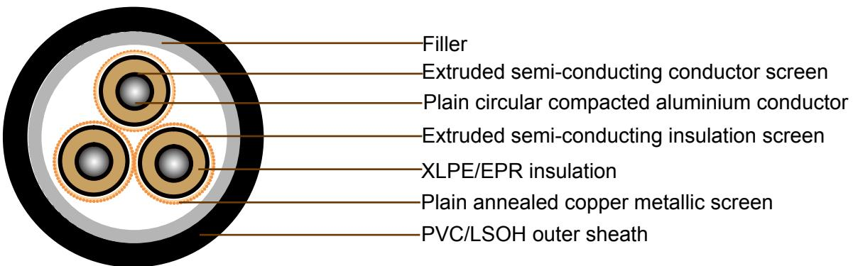
**CONDUCTOR:** Plain circular compacted aluminium to AS/NZS1125
