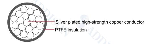
Conductor: Silver plated high-strength copper alloy
