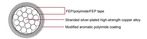
Conductor: Stranded silver-plated high-strength copper alloy conductor
