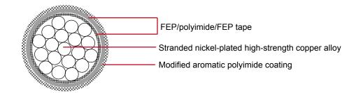
Conductor: Stranded nickel-plated high-strength copper alloy conductor
