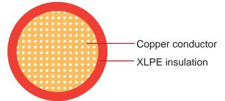
Conductor:Soft-annealed copper according to ASTM B
