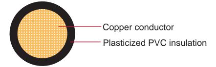
Conductor:Cu-ETP1 bare according to DIN EN 13602
