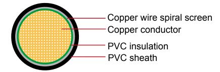
Conductor: Cu-ETP1 bare according to DIN EN 13602
