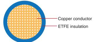
Conductor:Cu-ETP1 bare/tinned according to DIN EN 13602
