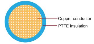
Conductor: Cu-ETP1 bare according to DIN EN 13602
