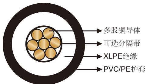
导体: ASTM B3和ASTM B8多股裸铜导体。
