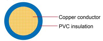
Conductor: Cu-ETP1 bare according to DIN EN 13602
